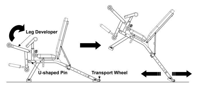
This incline bench has a pair of Transport Wheels on the rear stabilizer and can be carefully tilted onto its Transport Wheels for easy moving and storage. To move the bench, firmly grasp the Leg Developer with both hands and the Leg Developer must be locked by U-shaped Pin. Next, carefully pull the bench up until it rolls freely on the Transport Wheels.
